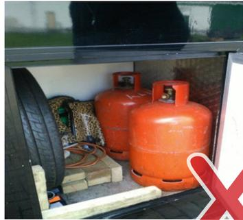
Cylinder compartment showing cylinders unrestrained in transit. Compartment also being used for storage of other items.
