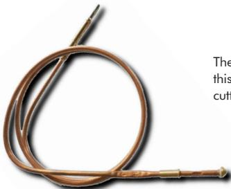
Thermocouple - when the heat is removed, this cools and causes a valve to close, cutting off the gas feed.
