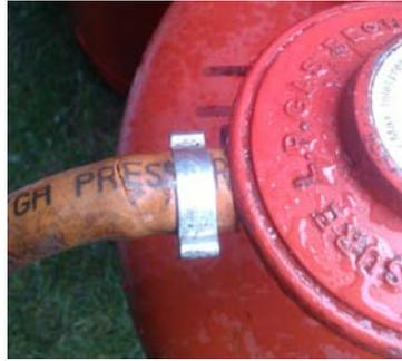
Damage to low pressure hosing leading from regulator.
