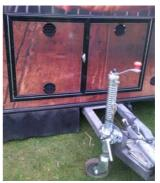
High and low level ventilation, in storage compartment door.
