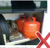
Cylinder compartment showing cylinders unrestrained in transit. Compartment also being used for storage of other items.
